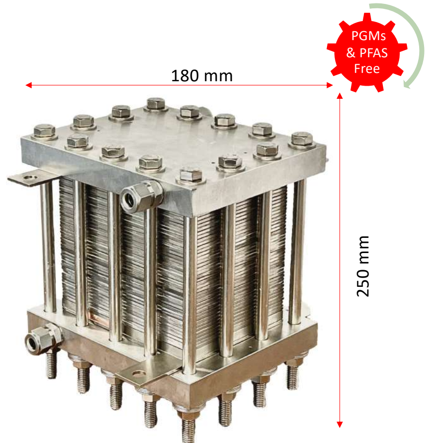
10 kW AEM Stack Hydrogen Production: 2000 liters/hour Pressure Range: 0 - 30 Bar
